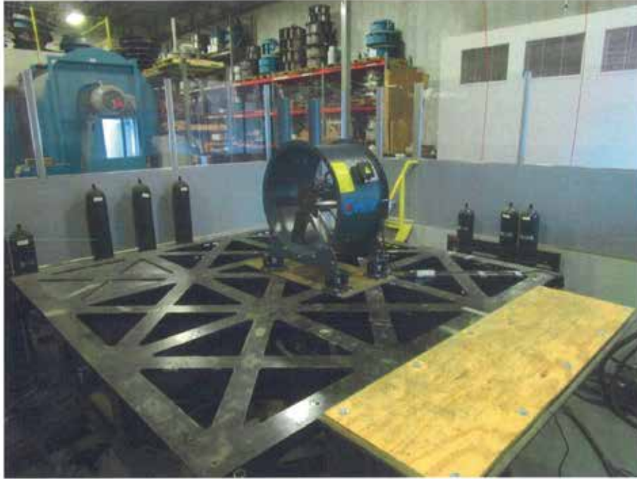
800mm Tubeaxial Seismic Test Setup
